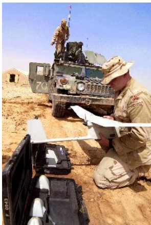
Army Corporal Jerry Rogers assembles a RQ-11 Raven unmanned aerial vehicle in order to conduct aerial tactical reconnaissance of insurgents in Taji, Iraq, on June 21, 2005. The Raven has video cameras located in the nose cone and can relay live video back to the operator in real-time. Rogers is attached to the Scout Platoon, 1st Battalion, 13th Armor Regiment, 3rd Brigade, 1st Armored Division. DoD photo by Tech. Sergeant Russell E. Cooley IV, U.S. Air Force. (Released)
